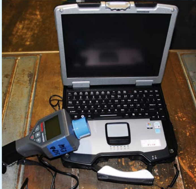
Radioisotope identification device (RIID) connected to a laptop. This unit can identify various radioactive isotopes. The spectra files can be downloaded onto a laptop computer that has the proper transfer software installed using either a serial cable or a USB cable.
